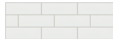
Shower Backsplash - Ceratec Essential - Bianco Glossy 4" x 16" -1/3 Offset Brick Lay Full Height Walls to Ceilings Mapei 5077 Frost Grout
