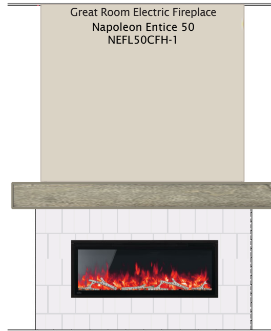
Fireplace Tile - Olympia Warm White Bright - 6 x 6 Installed 50/50 Brick with Frost Grout
