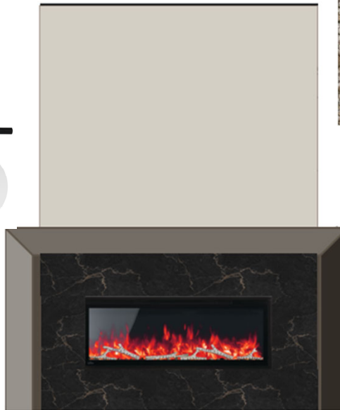
Fireplace Tile - Centura - Timeless - Nero Marquina Matte - 12 x 24 - Installed Horizontal Stacked with Charcoal Grout
