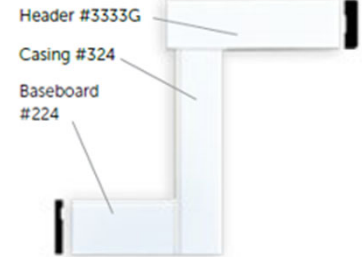
STANDARD - TRANSITION 3/4" x 3" - 14s #3333G 1/4" Rad MDF Header 3/8" x 3" - #324 MDF S/Bead Casing 1/2" x 4" - #224 MDF S/Bead Base
